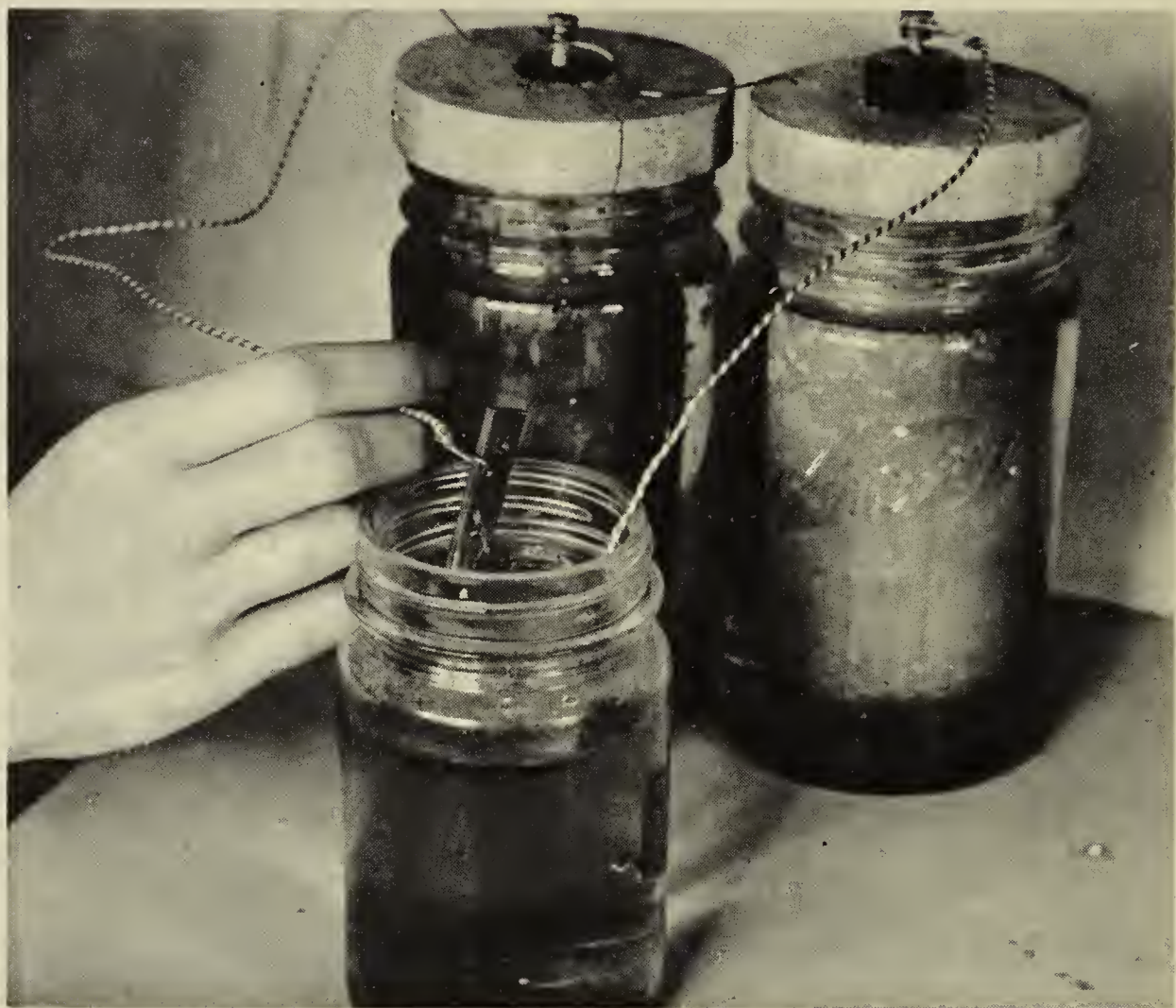
Fig. 18. Small brass objects can be electroplated with copper with this simple equipment.
